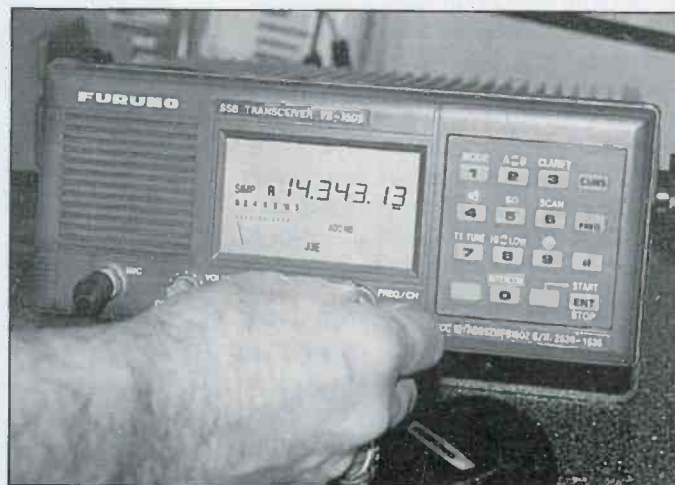
This Furuno high frequency marine SSB radio has continuous transmit and receive from 2 to 29.99 MHz.
