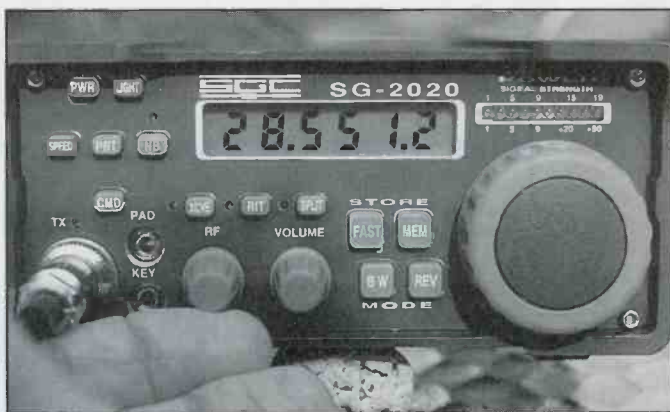
This little SGC sideband radio is already set for unlimited ham radio frequency coverage from 2 to 29 MHz!
