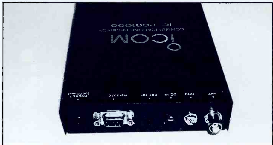
The computer-controlled receivers from ICOM, however, use their own protocol, and that includes a built-in interface. The cable is supplied, so you're all set with these receivers.
