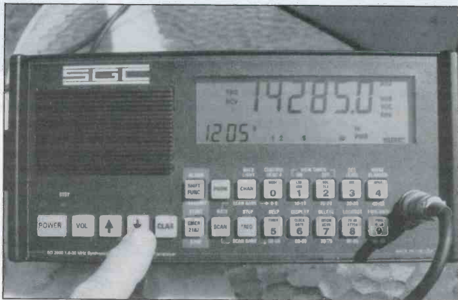
This S.G.C. marine SSB rig is already factory pre-programmed for ham radio use.
