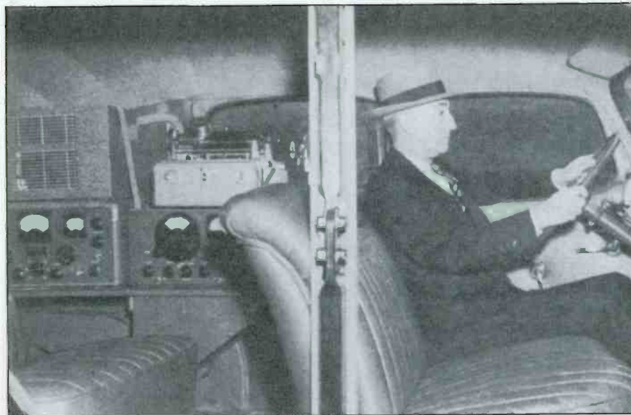
Side view of a FCC patrol unit engaged in the search for Fritz. This unit had two Hallicrafters receivers and a recorder that used aluminum alloy discs.
