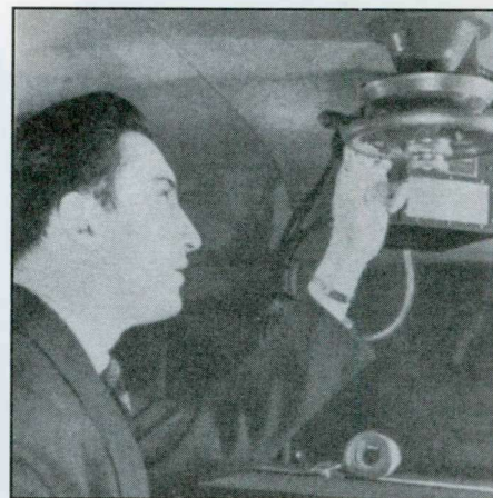
FCC mobile units had DF loops that could be rotated by hand.
