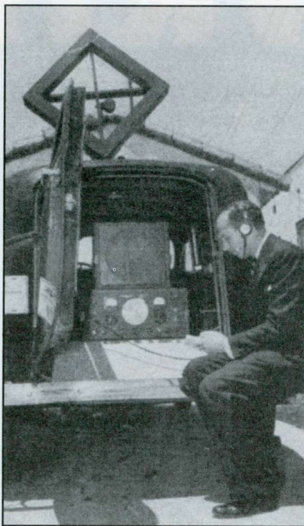
An FCC patrol unit equipped with a Hallicrafters SX-17 Super Sky rider takes DF bearings on Fritz.
