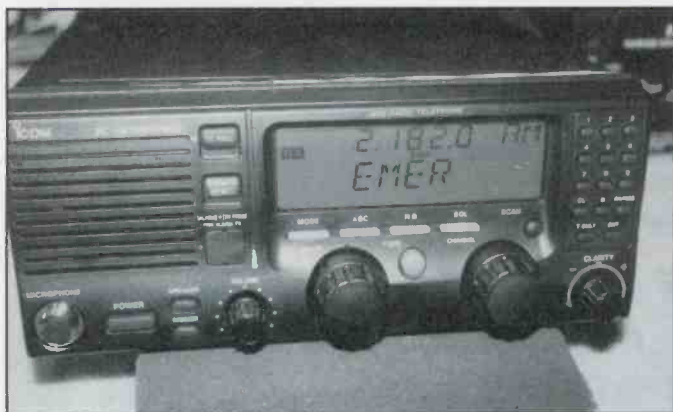
From ICOM is this powerful 150-watt marine SSB rig costing $1,400 new. It was sold for $300 at a marine swap meet. A computer upload turns it into a ham set.
